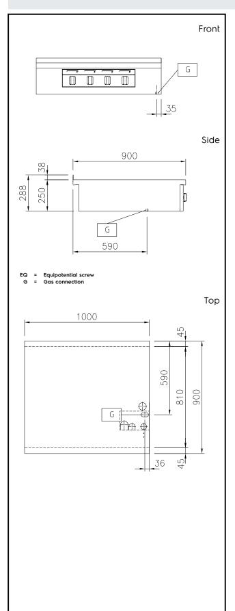
Gas Gas Power: 34 kW Gas Type Option: Gas Inlet: 1/2" **Key Information:** External dimensions, Width: 1000 mm External dimensions, Depth: 900 mm External dimensions, Height: 250 mm Net weight: 82 kg Configuration: One-Side Operated;Top Front Burners Power: 8.5 - 8.5 kW **Back Burners Power:** 8.5 - 8.5 kW **Back Burners Dimension -**Ø 70 Ø 70 mm
